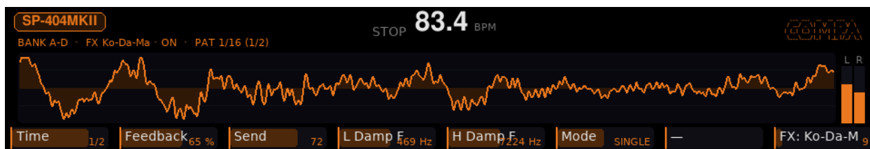
Push 2 — SP-404 Control with an active effect. Encoder labels relabel to the effect's parameter names.
