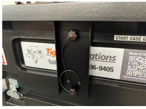
**STEP 3**: Place monitor arm through lid handle and attach with supplied tethered thumbscrews.
