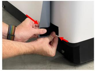
**STEP 5:** On the bottom edge, attach the end of the graphic to the velcro patch. Pull the two ends gently to provide tension and get a clean finished look.
